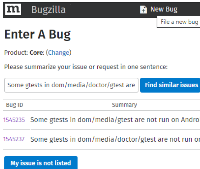
Figure 11. An example of the DBR retrieval feature in Bugzilla based on the bug summary.
